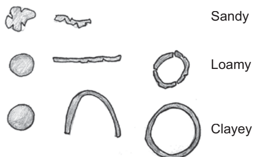
Figure 3.2. Method to determine soil the texture
