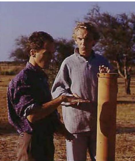
Piezometers: data from these could be crucial to the future of rice in the delta
